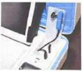
Verity Scan's vDrive/USE/Modern compartment, open, showing modern with USB connection and vDrive.
